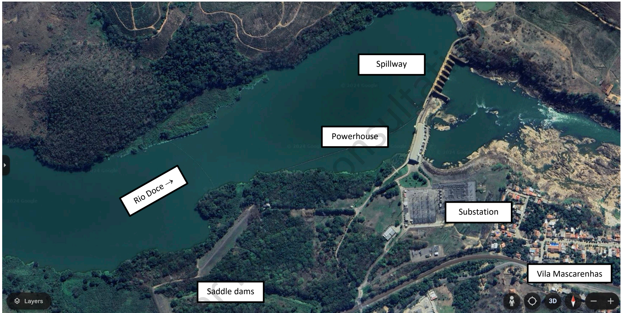
Figure 1 – Overview of Mascarenhas HPP, showing the Rio Doce flowing from left to right, the reservoir with its well-vegetated buffer zone, 2 saddle dams on the left bank, the main dam with a spillway on left, central dam, and powerhouse on right, the substation directly south of the powerhouse, the railway tracks (operated by mining company Vale S.A.), and the original village of Mascarenhas, which was expanded during construction of the HPP.
